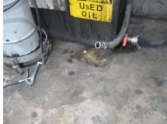
Release from used oil collector – Lawson space
